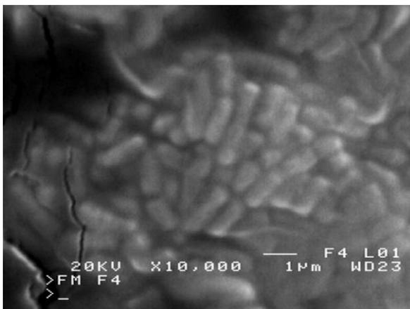
**Fig. 1.** Microcapsule surface image made by a scanning microscope. Enlargement 10 000×
