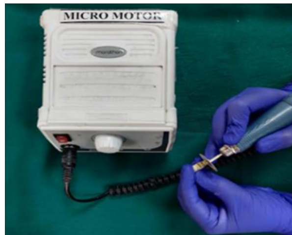
FIGURE 3. Specimen sectioning with diamond disks
