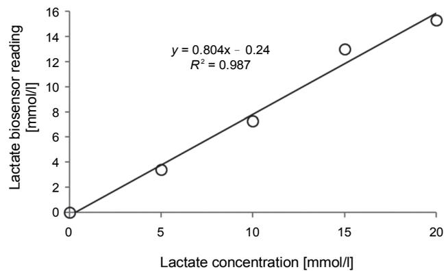
**Fig. 2.** The linearity of the lactate standard solution measured with the lactate biosensor at a temperature of 45°C
