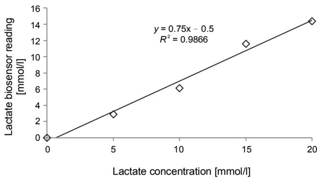
**Fig. 1.** The linearity of the lactate standard solution measured with the lactate biosensor at a temperature of 30°C
