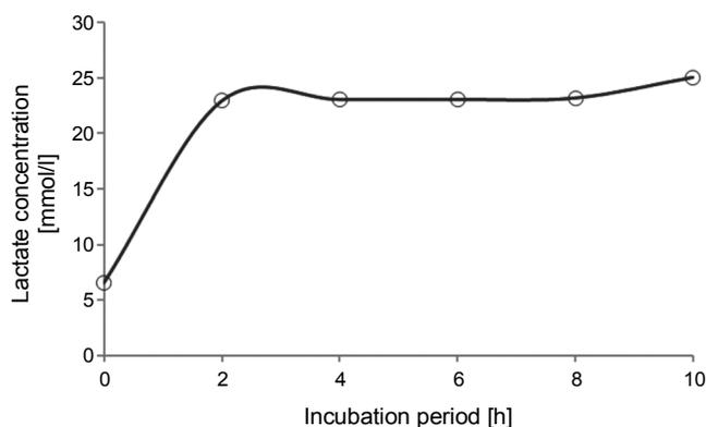
**Fig. 4.** Lactate concentration detected during the process of anaerobic acidification of taro starch
