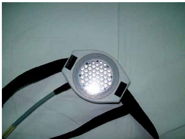
Figure 1. Elliptic magnetic–light applicator of Viofor JPS Light device applied for magneto-LED therapy procedures
