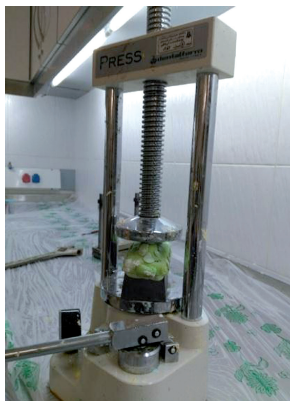
FIGURE 2. In vitro model with tray under pressing machine
