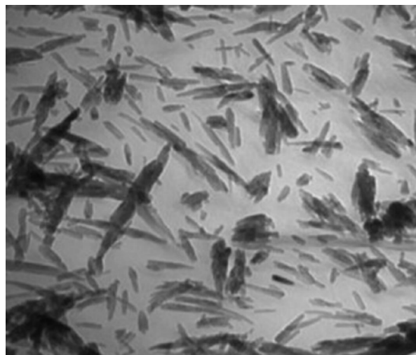
FIGURE 2. Transmission electron microscopy (TEM) images of the prepared nano-hydroxy apatite (n-HAP)
