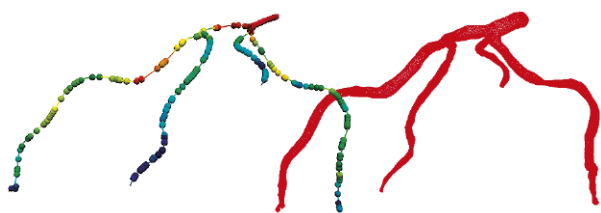
Fig. 3. Reconstruction of the central line and a final computational grid based on over 2 million finite elements
