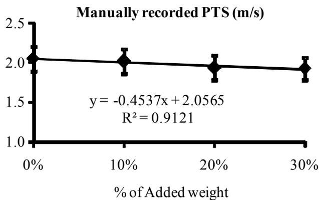
Figure 6. Manually recorded PTS decreased with the application of weight
