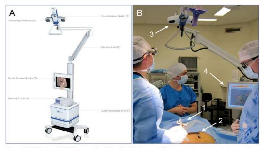
Figure 1: (A) Freehand SPECT system (SurgicEye, Munich, Germany) (B) Intraoperative setup and data acquisition using the freehand SPECT system with tracking targets on the gamma probe (1) and on the patient (2), which are monitored by the optical detection system (3), after which a reconstruction image can be displayed on screen (4).
